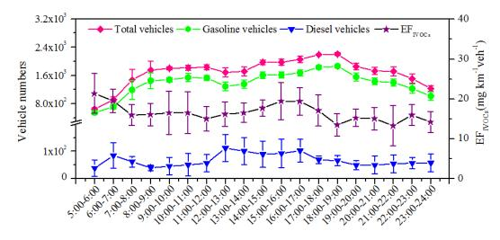
Figure 1. Diurnal variations of vehicle fleets and fleet-average  $EF_{IVOCs}$  during the sampling period. Error bars represent 95% confidence intervals.
