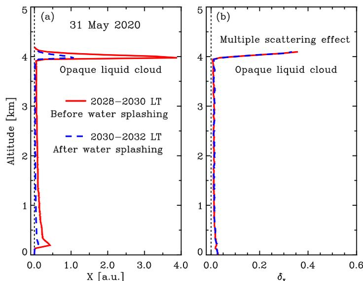
**Figure 1: Comparison of the lidar profiles with (integrated from 2030 to 2032 LT on 31 May 2020, dashed blue line) and without (integrated from 2028 to 2030 LT on the same day, solid red line) water accumulation on the lidar roof windows. (a), Range-corrected 355-nm signal  $X$  profiles; (b), 355-nm volume depolarization ratio  $\delta_v$  profiles. The water accumulation was produced by the artificial water splashing experiment.**
