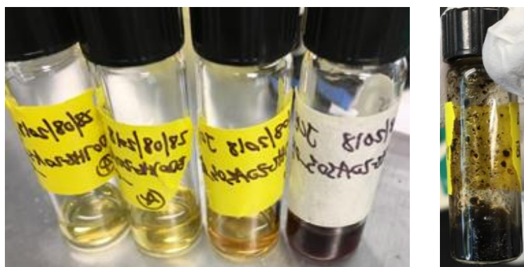
Figure S10. Series of 0.4 M BD/0.2 M AS solutions at increasing time of reaction rightward (left). 0.4 M BD/0.2 M AS solution after weeks of reaction (right). Solutions had approximately the same starting composition. The solutions darken over time and solids appear to form. A visible color change to a darker yellow was observed within minutes. Black-brown color was noticeable after hours of reaction. The accumulation of solids occurred on longer timescales (many hours to days). Solids were also observed rapidly (under an hour) in BD/NH x solutions with higher pH (e.g., in BD_NH_pH8.5 experiments).
