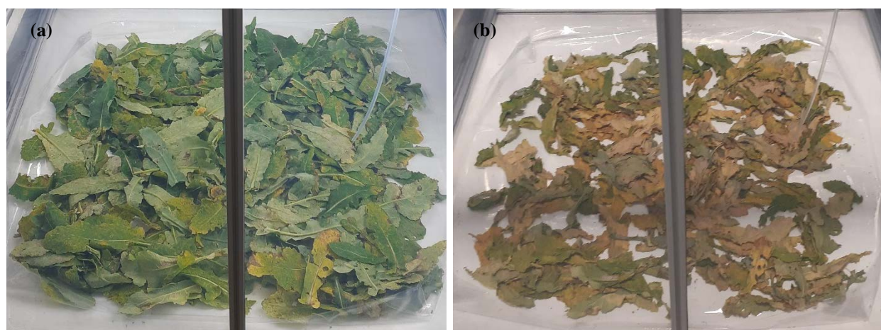
Figure 1: Example of the Rapeseed litter condition a) during the first day of the VOC and particles measurements and b) after 6 days of VOC and particles measurements.
