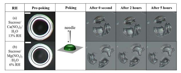
Figure 5. Optical images during poke-and-flow experiments at the points of pre-poking, poking, and post-poking for particles consisting of (a) sucrose/Ca(NO<sub>3</sub>)<sub>2</sub>/H<sub>2</sub>O particles and (b) sucrose/Mg(NO<sub>3</sub>)<sub>2</sub>/H<sub>2</sub>O particles for relative humidity (RH) where the particles shattered. The scale bar indicates 5  $\mu$ m.
