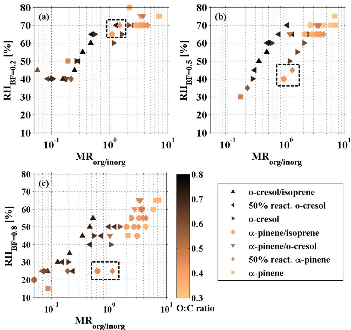
Figure 2. The measured (a)  $RH_{BF=0.2}$ , (b)  $RH_{BF=0.5}$  and (c)  $RH_{BF=0.8}$  as a function of organic-inorganic ratio ( $MR_{org/inorg}$ ) and coloured by atomic O:C ratio in various VOC systems photochemistry on deliquescent ammonium sulphate seed. Black box points out the  $RH_{BF=0.2}$ , 0.5, 0.8 at moderate  $MR_{org/inorg}$  of  $\sim 1$  for biogenic VOC systems ( $\alpha$ -pinene/isoprene, 50% reactivity  $\alpha$ -pinene).
