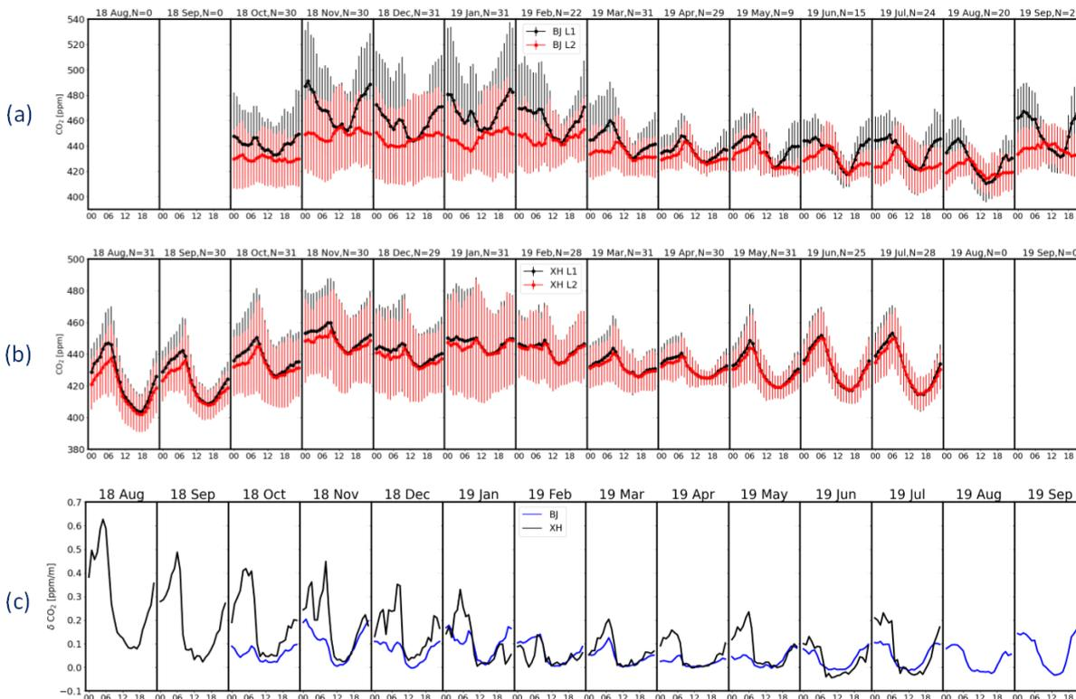
**Figure 10.** (a): the CO<sub>2</sub> measurements of BJ L1 and BJ L2 between October 2018 and September 2019. The error bars are the hourly standard deviations of CO<sub>2</sub>. (b): the CO<sub>2</sub> measurements of XH L1 and XH L2 between August 2018 and July 2019. (c): the hourly  $\delta$  CO<sub>2</sub> [ppm/m] in each month at BJ and XH.
