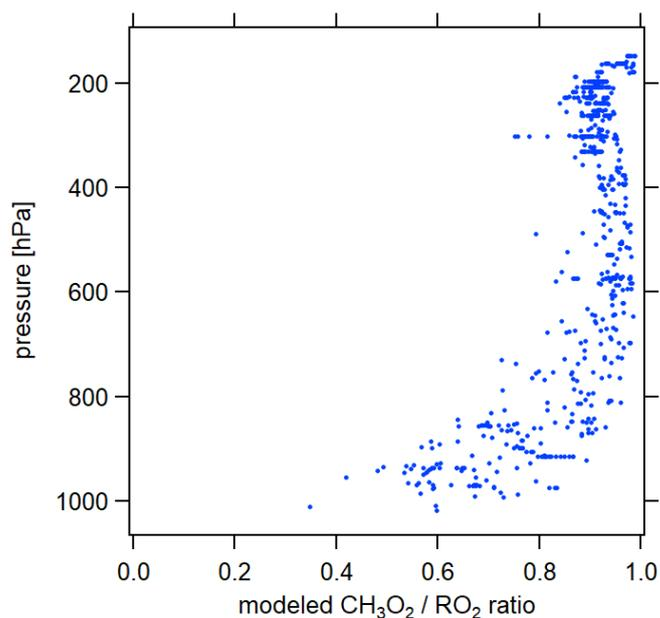
This figure shows the ratio of modeled CH<sub>3</sub>O<sub>2</sub> and RO<sub>2</sub> as a function of the pressure level for the BLUESKY campaign. It can be seen that above 800hPa, CH<sub>3</sub>O<sub>2</sub> represent > 90 % of the overall modeled RO<sub>2</sub>. In the lower troposphere CH<sub>3</sub>O<sub>2</sub> accounts for on
