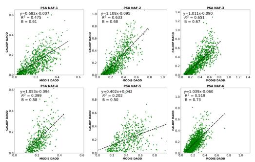
Figure 9. Comparison of CALIOP DAOD against MODIS DAOD over six dust aerosol source regions in North Africa from NAF-1 to NAF-6 as indicated in Figure 8. The mean bias (B) is computed as the average of CALIOP DAOD / MODIS DAOD ratios of all data pairs. B = 1, >1, <1 indicates no bias, high bias and low bias.
