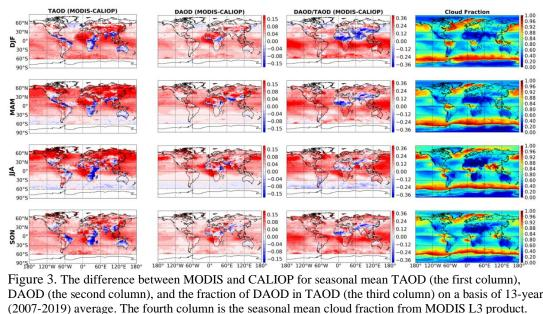
Figure 3. The difference between MODIS and CALIOP for seasonal mean TAOD (the first column), DAOD (the second column), and the fraction of DAOD in TAOD (the third column) on a basis of 13-year (2007-2019) average. The fourth column is the seasonal mean cloud fraction from MODIS L3 product.
