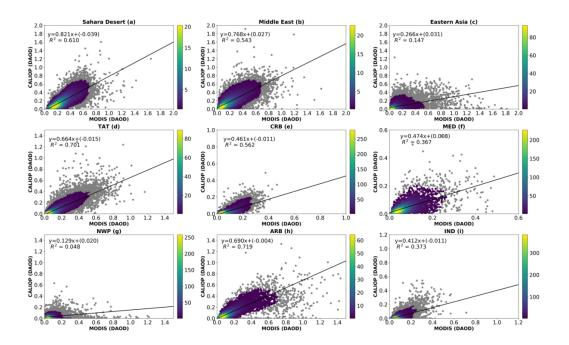
Figure 5. Comparison of CALIOP DAOD against MODIS DAOD over dust-laden regions indicated in Figure 4. Color represents the probability density using gaussian kernel density estimation. Grey points represent data points within the lowest 5% of data density. Those grey points are excluded in the linear regression analysis.
