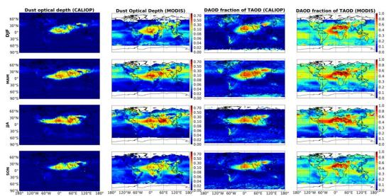
Figure 1. Spatial distribution of the seasonal mean CALIOP-based DAOD, MODIS-based DAOD and the fraction of DAOD with respect to the TAOD based on CALIOP and MODIS respectively for the globe at a 5° *longitude* × 2° *latitude* resolution based on 13-year (2007-2019) CALIOP measurements. **DJF**: December from previous year-January-February; **MAM**: March-April-May; **JJA**: June-July-August; **SON**: September-October-November.
