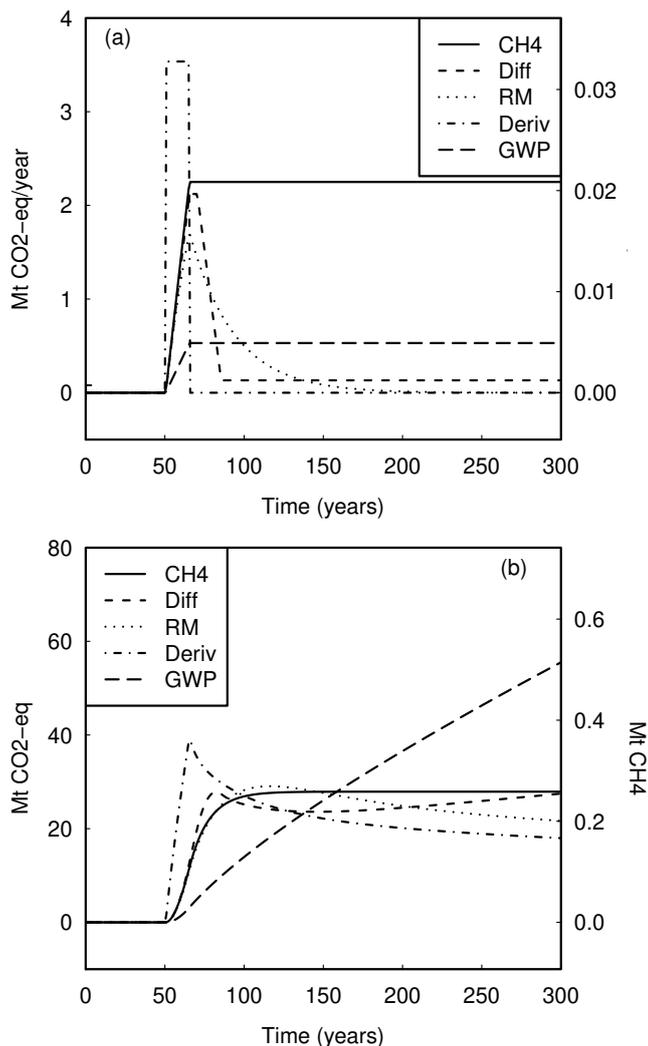
(b) CH<sub>4</sub> concentrations from source shown in Figure 6 part (a) (solid line) and the CO<sub>2</sub> concentrations resulting from the CO<sub>2</sub> concentrations resulting from the equivalent CO<sub>2</sub> sources, as shown in Figure 6 part (a). The relative scaling of the axes is  $a_{CH_4}/a_{CO_2}$  so that the radiative forcing can be compared directly.
