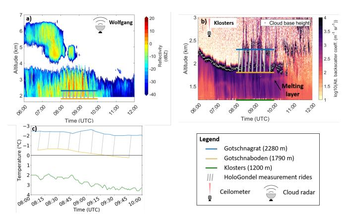
**Figure 3.** Observations of the reflectivity measured by the cloud radar installed in Wolfgang are shown in a). The ceilometer data in b) shows the estimated cloud base with grey dots above Klosters. A dark band underneath the cloud base indicates the melting layer. Temperature measurements at the Gotschnagrat, the Goschnaboden and Klosters, during the time HoloGondel was measuring, are shown in c).
