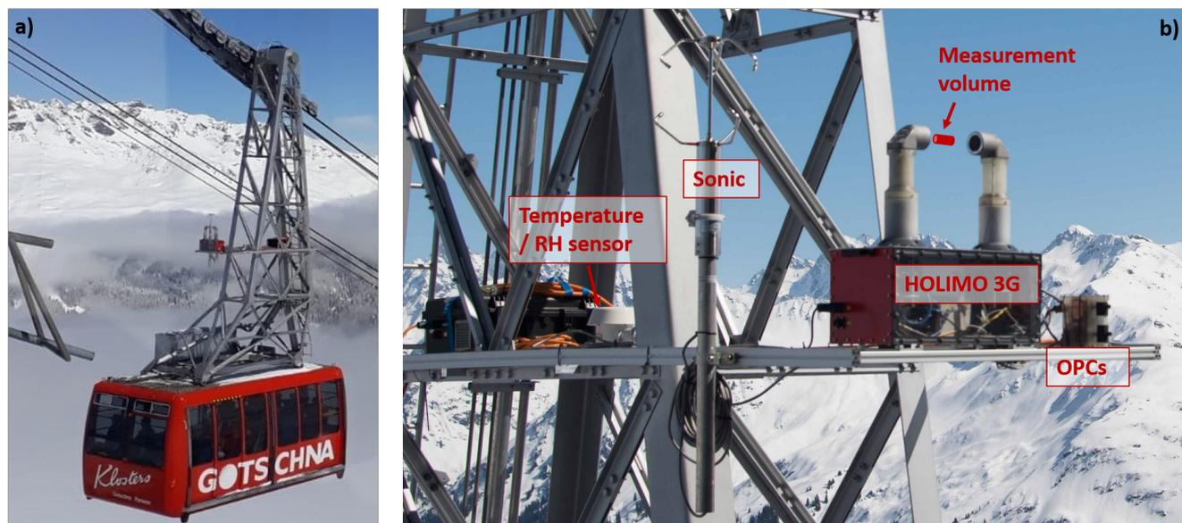
**Figure 2.** The HoloGondel platform installed on the Gotschnabahn in a) and an enlarged picture of the platform in b) showing HOLIMO 3G with its measurement volume between the two towers, two optical particle counters (not used in this study) next to HOLIMO and the temperature / RH sensors. The Sonic anemometer was turned off due to a limited supply of power.
