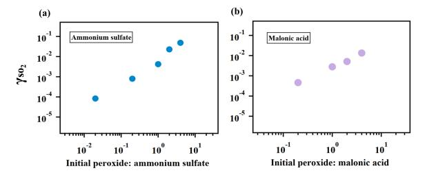
**Figure 3.** Relationship between  $\gamma_{SO2}$  and particulate peroxide content.  $\gamma_{SO2}$  for ammonium sulfate (a) and malonic acid aerosol (b) containing different amount of 2-butanone peroxide are shown here. The observed dependence of  $\gamma_{SO2}$  on the amount of peroxide injected are linear since the slopes of the relationship are both nearly 1 in (a) and (b).
