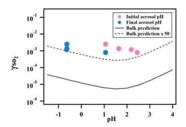
**Figure 5.** Relationship between  $\gamma_{SO2}$  and aerosol phase pH for ammonium sulfate aerosol containing 2-butanone peroxide.
