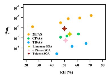
**Figure 6.**  $\gamma_{SO2}$  measured for different types of organic aerosol. The reactive uptake coefficient of  $SO_2$  onto SOA are on the order of  $10^{-4}$ .
