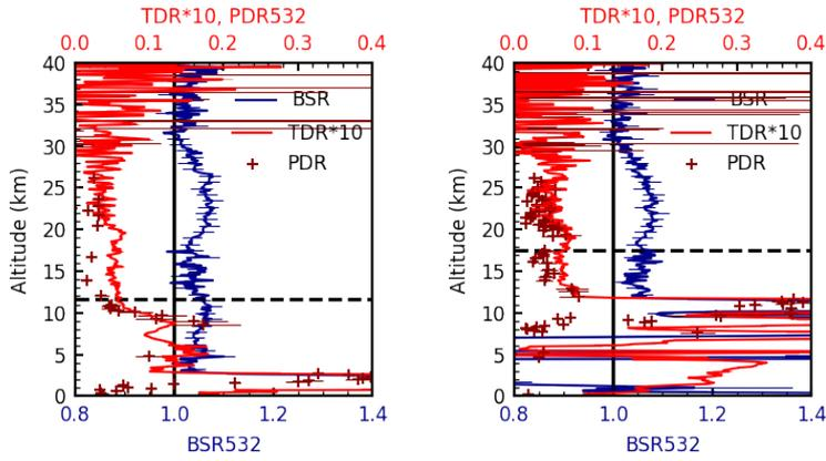
Figure R3-1. Lidar profiles taken at Tsukuba on May 2, 4, 10, 13, 14, 15, 18, 19, 22, 24, and 28, 2018. The horizontal dashed line in each panel indicates the location of the first lapse rate tropopause. It is noted that for “TDR\*10” = 0.05 means  $TDR = 0.05/10 = 0.005$ , i.e., 0.5%TDR. This is close to the depolarization ratio value, 0.366% for air molecules.
