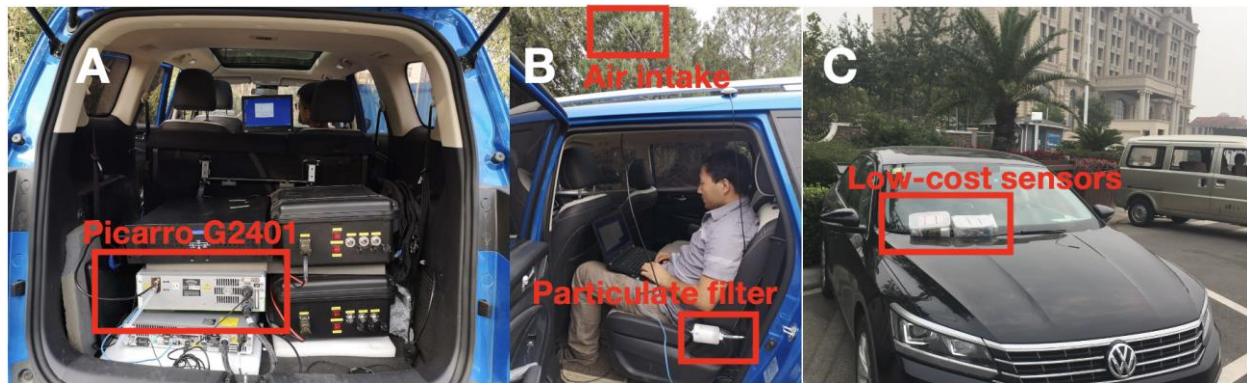
Figure 2. Photographs of the instrument installation for the on-road observations. (A) and (B) Picarro system installed in the vehicle; (C) low-cost non-dispersive infrared (NDIR) sensors installed on the front windshield of the vehicle.
