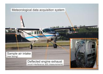
**Figure 2.** The DLR Cessna 208B on the taxiway at Katowice airport. The sample air intake is mounted underneath the right wing. The meteorological data acquisition system underneath the left wing. The QCLS instrument (lower left panel) is located inside the cabin behind the pilot seats.
