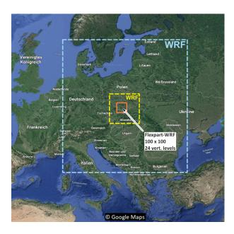
**Figure 3.** The FLEXPART-WRF domain resides in the nested WRF domain D2 providing the meteorological driver data. Generous spacing towards the driver domain has been included to avoid spurious boundary effects.
