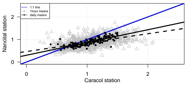
**Figure 10.** Comparison of the SO<sub>2</sub> emission flux estimates when both NOVAC stations observed volcanic plumes within the same time bin of hourly means (grey triangles) and daily means (black circles). Data compares the bin averages and only data for wind speeds larger than 5 m/s were considered.
