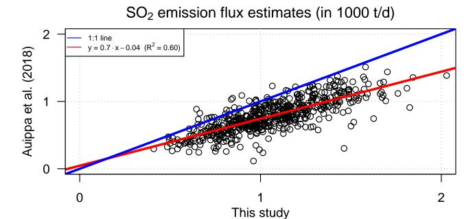
Figure 12. Comparison of the SO<sub>2</sub> emission fluxes from Caracol station reported in this study and by Aiuppa et al. (2018).
