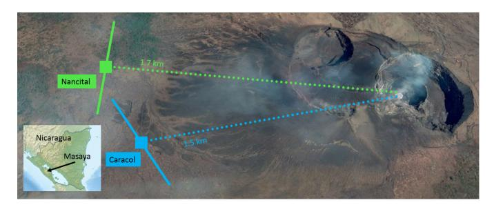
Figure 1. Location and scan geometries of the NOVAC stations Caracol and Nancital at Masaya volcano. Coloured squares indicate the location and solid lines the scan direction. For further parameters see Table 1. The map was created with graphical material from https://commons.wikimedia.org/wiki/File:Nicaragua\_relief\_location\_map.jpg and from © Google Earth.
