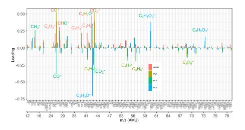
**Figure 3.** Loadings of the first three principal components and the normalized mean AMS mass spectrum (shown up to m/z 80). Fragment ions with high positive/negative loadings are indicated by their formula and are color-coded for each PC.
