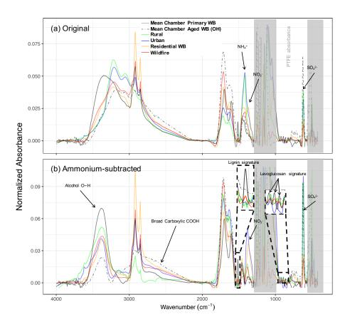
**Figure 6.** Normalized (Euclidean norm) mean spectra of ambient aerosols (rural, urban, residential wood burning, and wildfire) and chamber WB aerosols before (a) and after subtraction of ammonium profile (b). Inorganic nitrate and sulfate absorbances still exist in panel (b).
