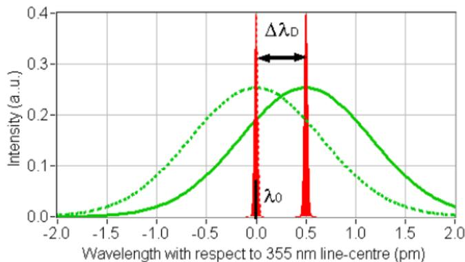
**Figure R1.** Wavelength spectra for the backscattered Mie (red) and Rayleigh (green) signal for a 355 nm source at  $\lambda_0$  (dotted lines) and a Doppler shift  $\Delta\lambda_D$  (bold lines); the indicated Doppler shift of 0.5 pm corresponds to a LOS wind speed of  $\sim 200 \text{ ms}^{-1}$
