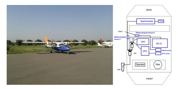
**Figure 4.** Piper PA 34 Seneca aircraft (left panel) and the schematic of the aerosol inlet and sampling instruments inside the plane (right panel). Aerosol sampling lines are shown in black and sampling instruments in blue.
