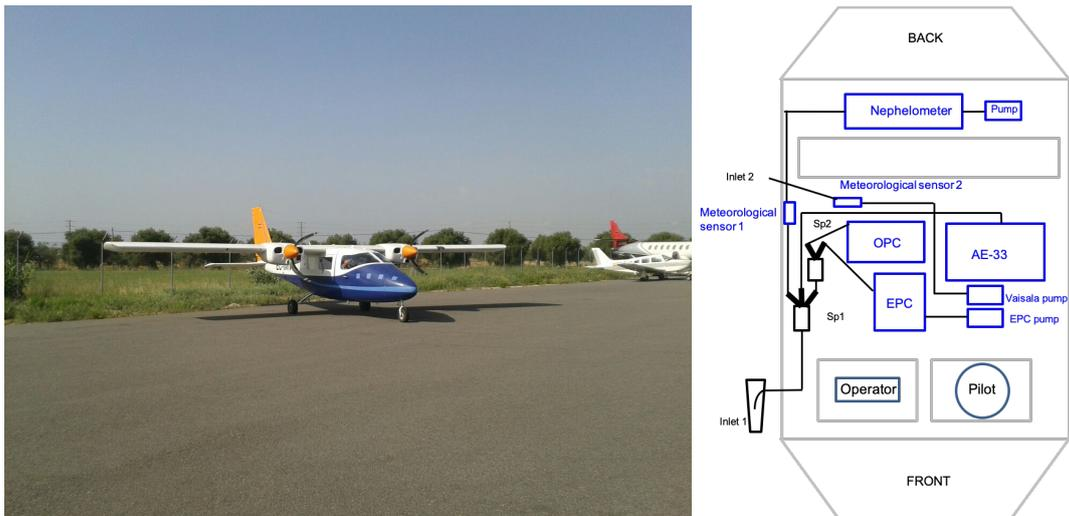
**Figure 4.** Piper PA 34 Seneca aircraft (left panel) and the schematic of the aerosol inlet and sampling instruments inside the plane (right panel). Aerosol sampling lines are shown in black and sampling instruments in blue.
