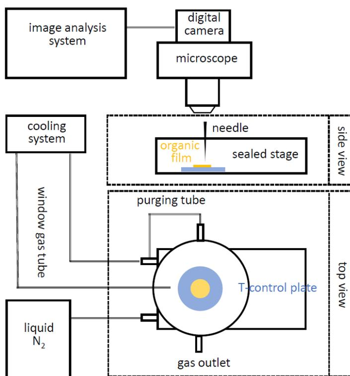
**Figure 2.** Schematic of the experimental poke-flow setup. This includes a temperature controlled Linkam cooling stage coupled to a microscope equipped with a digital camera and an image analysis system.
