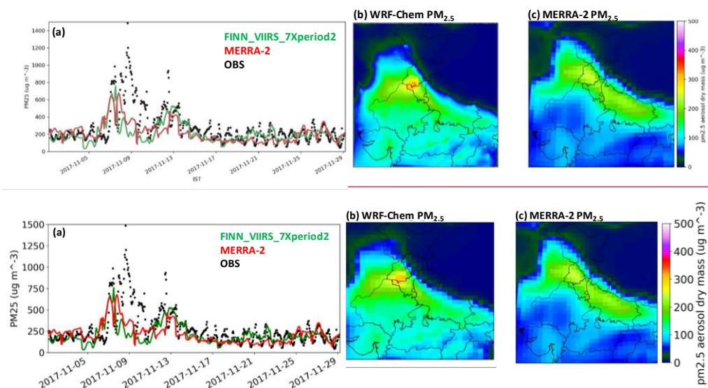
**Figure 5** Temporospacial air quality performance of base scenario simulation: a) Time series of simulated (green line), MERRA-2 (red line), and ground measurement (black dots) hourly PM<sub>2.5</sub> concentration at US Embassy coordinates. b, c) Hourly averaged PM<sub>2.5</sub> concentration maps of model regridded to MERRA-2 resolution (b) and MERRA-2 (c).
