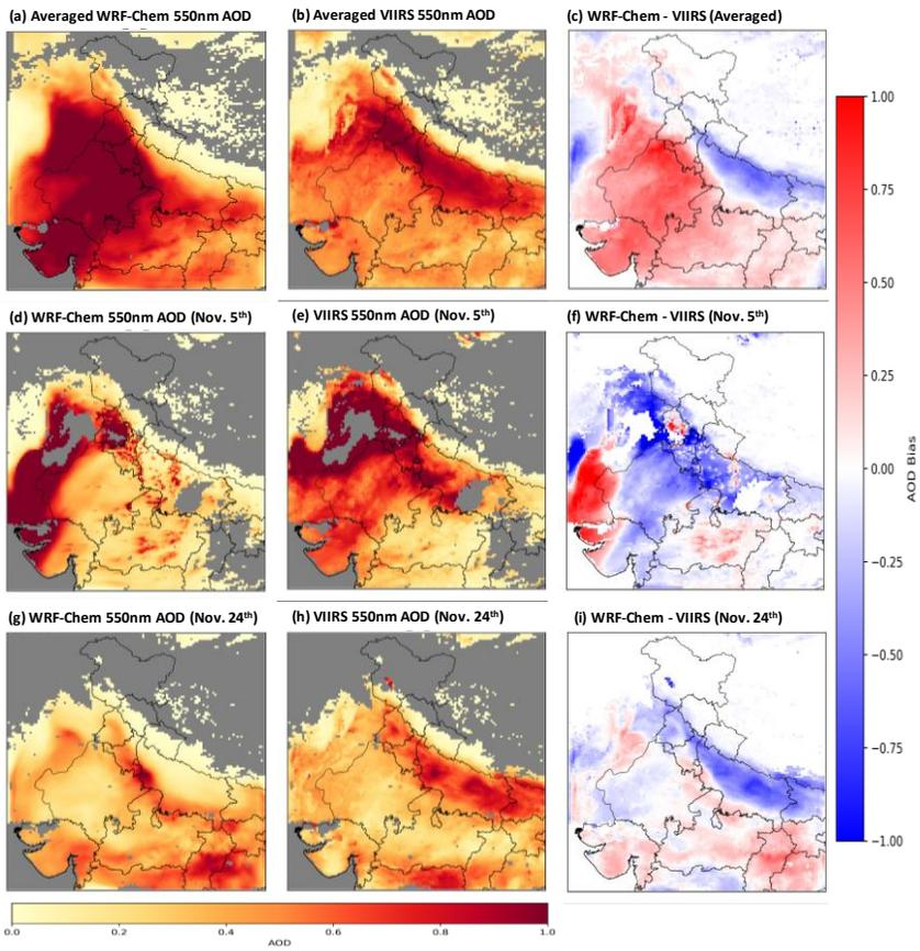
390 **Figure 3** Spatial distributions of AOD at 550 nm averaged over whole November (top panel), Nov. 5<sup>th</sup> (middle panel), and Nov. 24<sup>th</sup> (bottom panel). WRF-Chem maps represent base scenario results. Differences between model and VIIRS are also shown.
