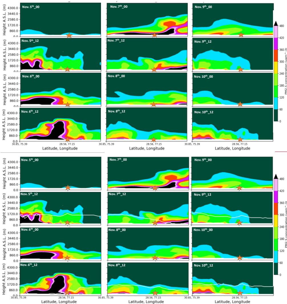
470 **Figure 8** Vertical cross section of PM<sub>2.5</sub> concentration through the path shown in Fig. 1 for the days between Nov. 5<sup>th</sup> and Nov. 10<sup>th</sup>. For each day, two snapshots are shown at 00UTC (5:30AM local time) and 12UTC (5:30PM local time). The orange star shows the location of Delhi through the path. White line shows the PBL height across the path.
