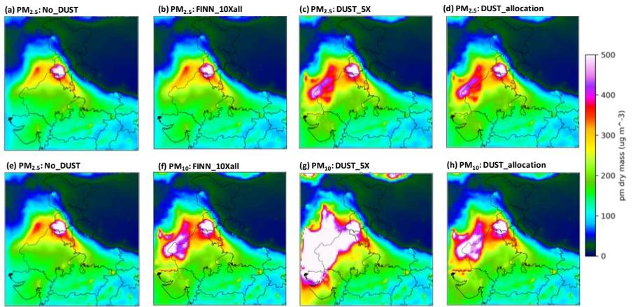
**Figure 15** Responses of  $PM_{2.5}$  and  $PM_{10}$  to changes in dust emissions: a, e) dust is turned off, b, f) dust is turned on, c, g) dust emissions are increased by 5 times, and d, h) dust emissions with different allocation in MOSAIC bins.
