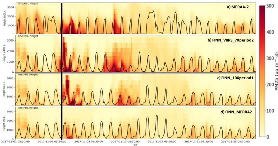
**Figure 1243** Vertical cross section of  $PM_{2.5}$  sensitivity to major changes in FINN emission inventory at US Embassy coordinates: a) MERRA-2 data as true values, b) FINN\_VIIRS\_7Xperiod2, c) FINN\_10Xperiod, d) FINN\_MERRA2. Black lines present planetary boundary layer height. Vertical black line crossing all panels shows boundary layer peak on Nov. 6<sup>th</sup> for MERRA-2 and other experiments.
