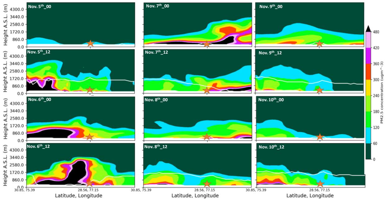
Figure 7 Figure 8 Vertical cross section of  $PM_{2.5}$  concentration through the path shown in Fig. 1 for the days between Nov. 5<sup>th</sup> and Nov. 10<sup>th</sup>. For each day, two snapshots are shown at 00UTC (5:30AM local time) and 12UTC (5:30PM local time). The orange star shows the location of Delhi through the path. White line shows the PBL height across the path
