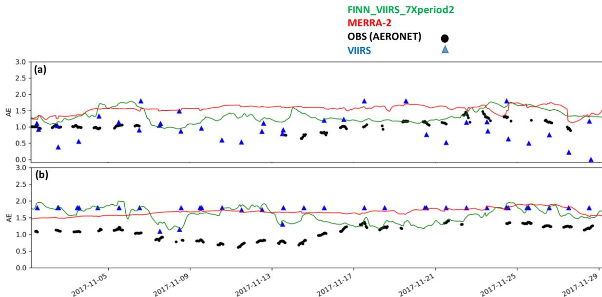
Figure 4 Time series of modeled (green line), VIIRS retrievals (blue triangle), MERRA-2 (red line), and AERONET (black dots) Angstrom Exponent during Nov. 2017 at a) Jaipur, b) Kanpur.
