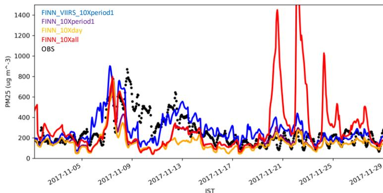
**Figure 10** Time series of model PM<sub>2.5</sub> sensitivity to 10 times increase in FINN emission inventory for different periods: FINN\_VIIRS\_10Xperiod1: Nov. 3<sup>rd</sup> to 17<sup>th</sup>, FINN\_10Xperiod1: Nov. 3<sup>rd</sup> to 17<sup>th</sup>, FINN\_10Xday: Nov 5<sup>th</sup>, FINN\_10Xall: all days. Black dots presents ground measurements data averaged over all CPCB stations in Delhi.
