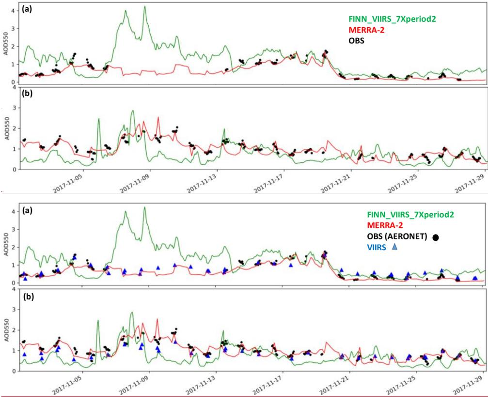
**Figure 4** Time series of modeled (green line), VIIRS retrievals (blue triangle), MERRA-2 (red line), and AERONET (black dots) AOD at 550 nm during Nov. 2017 at a) Jaipur, b) Kanpur.
