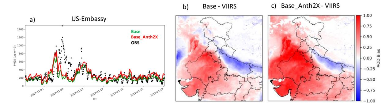
Figure 1 a) Timeseries for PM<sub>2.5</sub> concentration at the location of US embassy using Base scenario and Base\_Anth2X scenario b) Bias of AOD at 550nm averaged over November 2017 based on b) base scenario c) base scenario with 2 times more anthropogenic particle emissions (ID: Base\_Anth2X)
