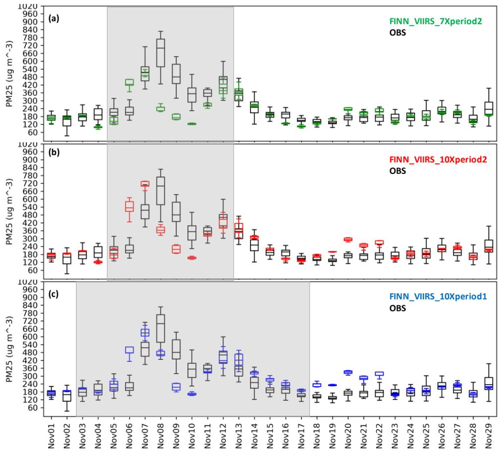
**Figure 6** Box and Whisker plots of observed (black) and modeled daily PM<sub>2.5</sub> concentration averaged over all CPCB stations in Delhi: a) FINN\_VIIRS\_7Xperiod2, b) FINN\_VIIRS\_10Xperiod2, c) FINN\_VIIRS\_10Xperiod1. Shaded area show the time window that biomass burning emissions were increased.
