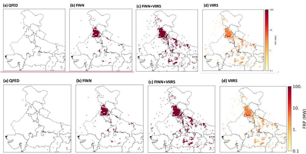
510 **Figure 9** Spatial fire coverage in different datasets for Nov. 5th: a) QFED fire grid cells b) FINN fire grid cells c) FINN fire grid cells filled missing points with VIIRS d) VIIRS active fire points and corresponding FRP values.
