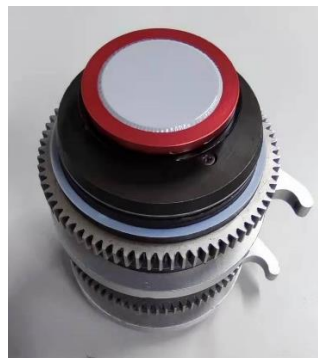
Figure R2.1. Photograph of a collection plate fixed with a polycarbonate filter
