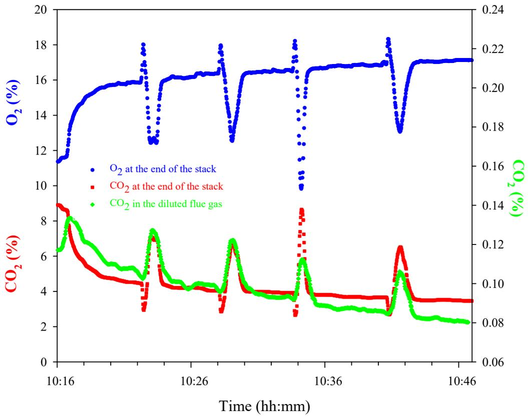
Figure 2 Example (PS-F9 sample) for the variations of the measured CO<sub>2</sub> and O<sub>2</sub> mixing ratios at the end of the stack and the CO<sub>2</sub> mixing ratio in the diluted flue gas during combustions tests.
