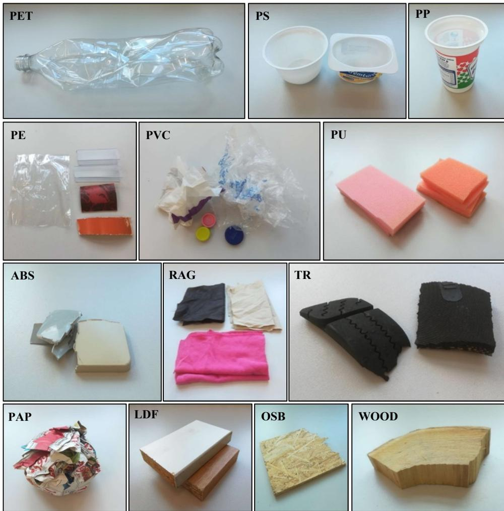
Figure 1 Solid waste specimens prepared for combustion tests.
