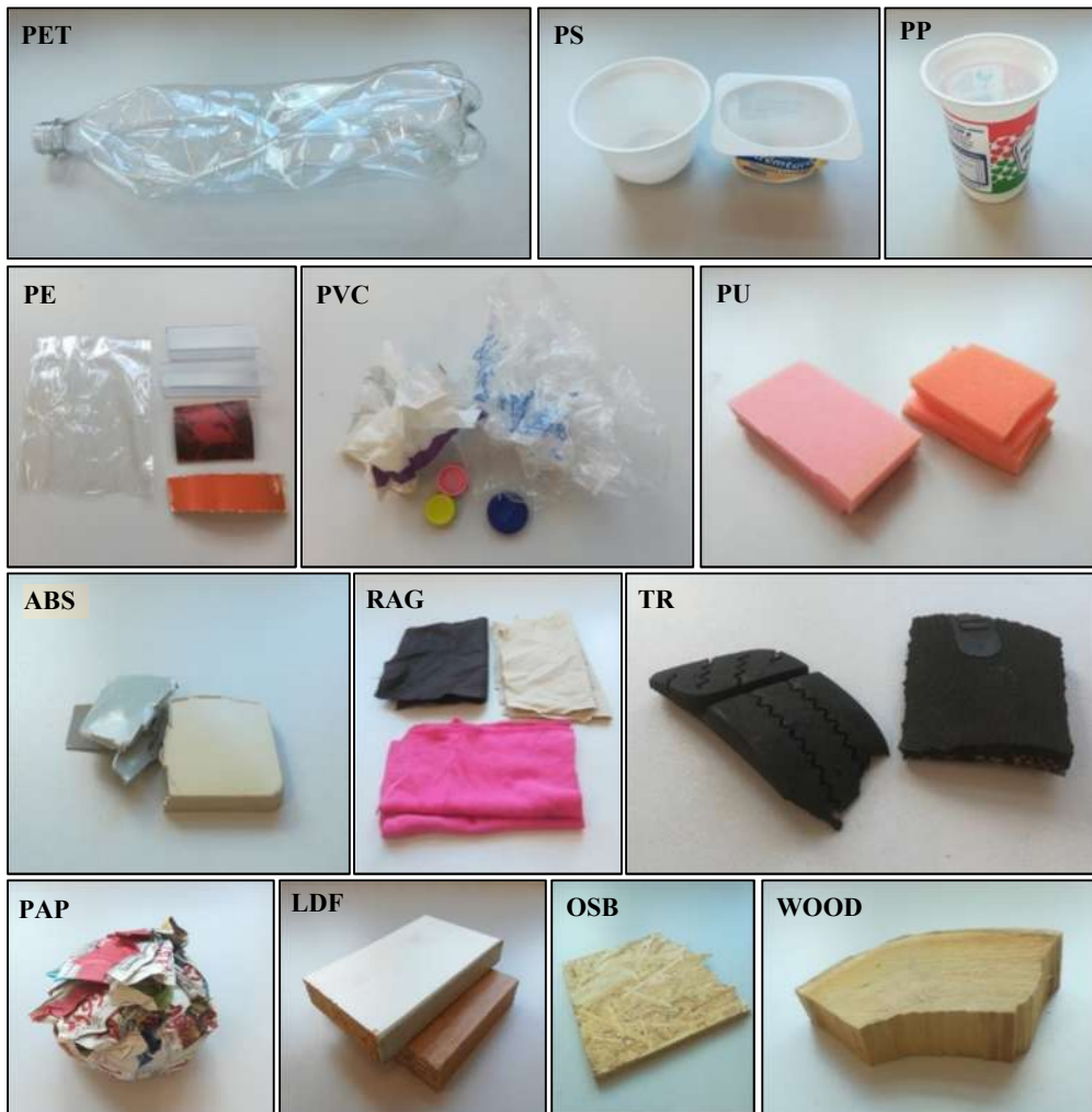
Figure 1 Solid waste specimens prepared for combustion tests.
