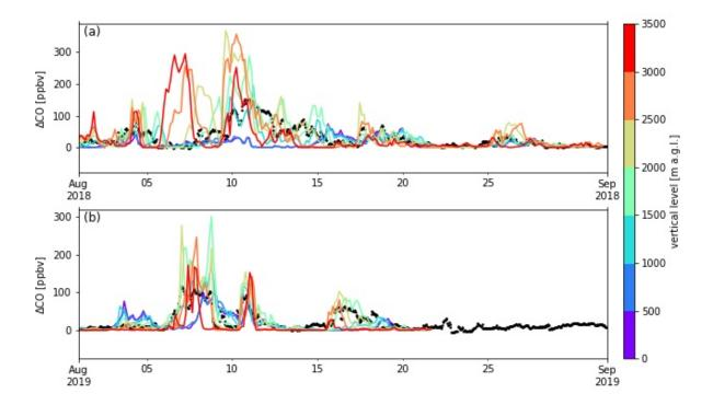
**Figure 4.** Comparison between measured excess CO (black) at RUN to that modelled on different vertical levels of the FLEXPART model during August 2018 (a) and August 2019 (b). FLEXPART output levels are defined in meters above ground level (m a.g.l.).
