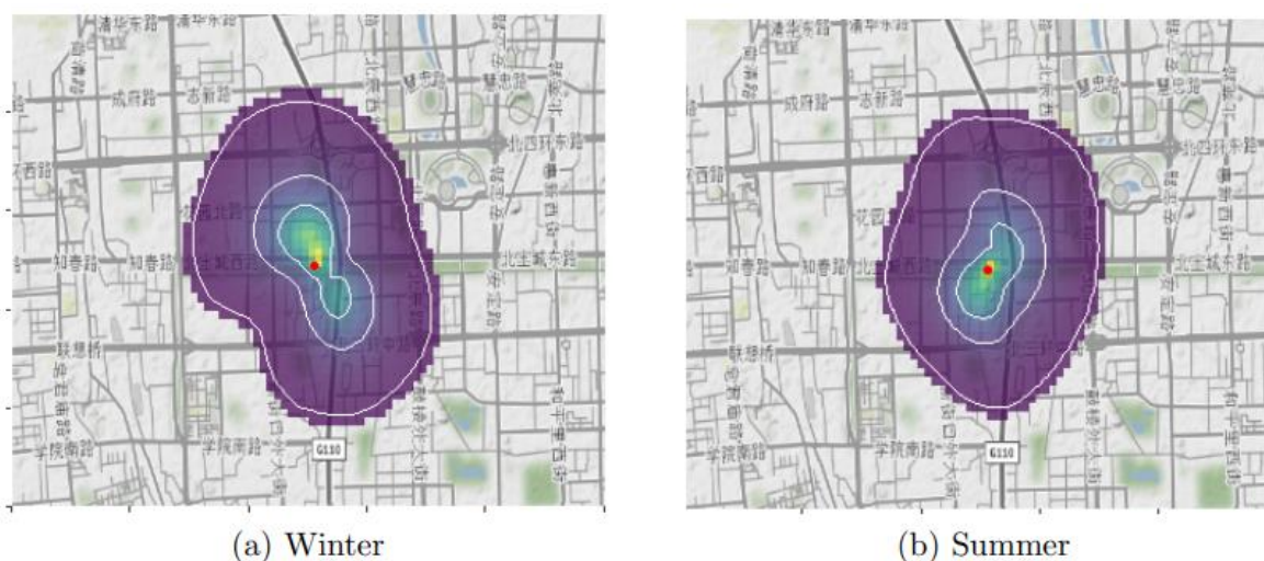
Figure 7. Total average mass flux footprints for winter and summer seasons. The red spot on each plot is the location of the IAP tower, and surrounding colours represents the magnitude of the intensity of the measured emission. The resolution of footprint is 100 \text{ m}^2 , the outermost white line represents the 90% cumulative spatial contribution of the total flux and the middle and inner most lines representing 60% and 30% contribution. Map tile sets are © Stamen Design, under a Creative Commons Attribution (CC BY 3.0) license.
