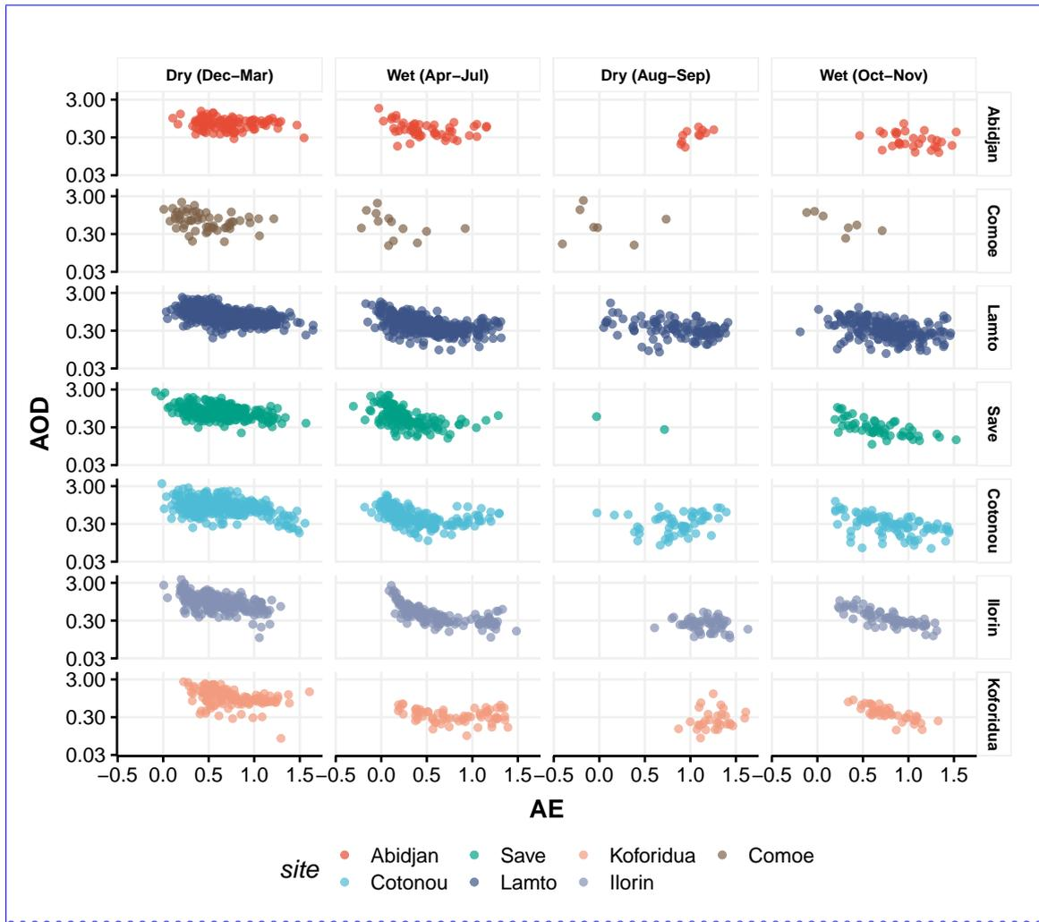
Figure 7. Scatter plots of sun photometer aerosol optical depth (AOD) versus Ångström exponent (AE) splitted by sites and by seasons.
