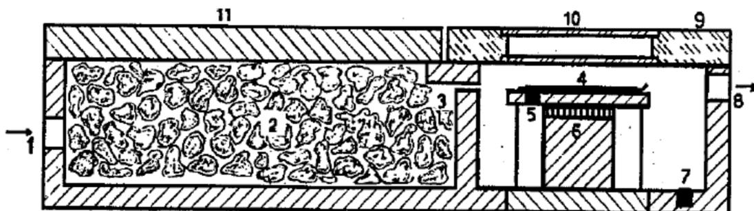
**Figure.** 1: air inlet; 2: minced ice; 3: slit and air temperature thermocouple; 4: filter; 5: filter temperature thermocouple; 6: Peltier cooling device; 7: thermocouple; 8: air outlet; 9: plexiglass cover; 10: observation slit.
