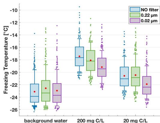
685 Figure 5. Freezing temperature boxplots for the size filtration series. Aqueous lignin solutions of  $200 \text{ mg C L}^{-1}$  and  $20 \text{ mg C L}^{-1}$
