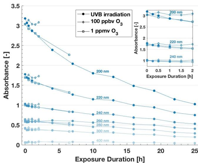
700 Figure 7. Wavelength-specific absorption values from UV/Vis spectra of 20 mg C L<sup>-1</sup> lignin solutions after atmospheric processing through UVB irradiation and exposure to O<sub>3</sub>. The insert is a zoom of the plot section from 0 to 2 h exposure duration. With increasing exposure duration, lignin's absorbance is decreasing. Changes after exposure to 100 ppbv O<sub>3</sub> are minimal.
