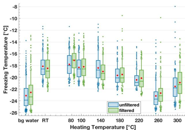
690 Figure 6. Freezing temperature boxplots of the  $200 \text{ mg C L}^{-1}$  lignin solutions directly after heating (blue, unfiltered) and after
