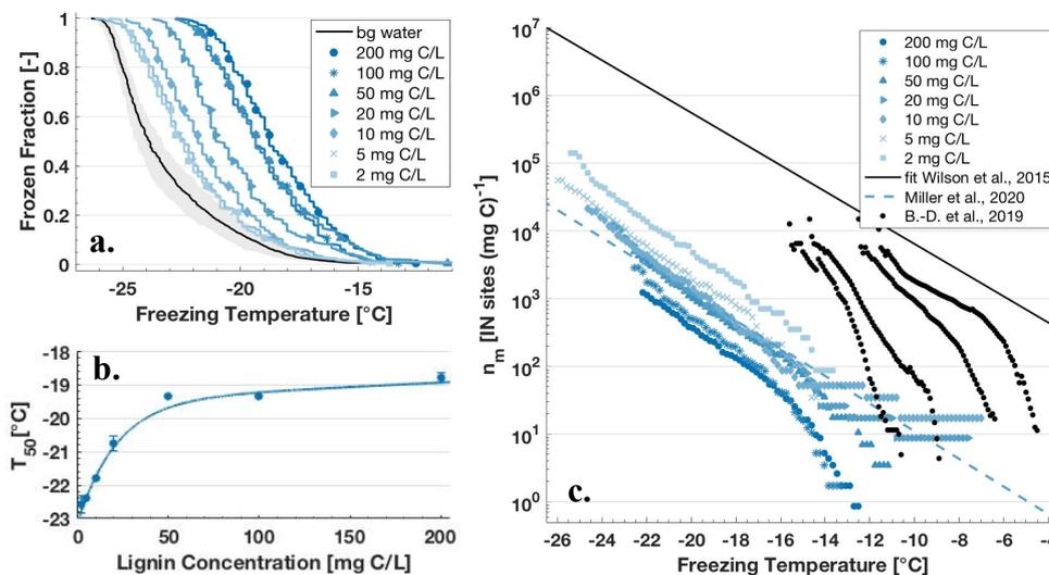
675 Figure 4: (a) Freezing temperatures for aqueous dilution series as FF curves. The FF curves include the water background (bg water
