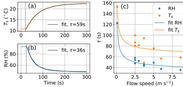
**Figure A1.** Time response of the humidity sensor to a step function experiment: (a) sensor-internal temperature  $T_s$  and (b) RH at  $8.6 \text{ m s}^{-1}$  with fitted time constants  $\tau$ . Panel (c) shows the time constants depending on the flow speed. A root fit function is added to the values.
