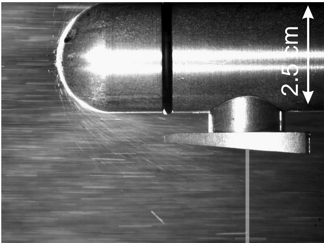
900 Figure 15. A snapshot from a high-speed video showing a flow of shattered ice fragments rebounding from the hemispherical tip of the OAP-2DC particle probe. The shattered ice fragments deflected toward the sample area (bright vertical band) are counted by the probe and artificially enhance the measured concentration. The video recording was performed in an ice spray at 80m/s in the Cox and Co. Icing Wind Tunnel Facility (for more details see Korolev et al. 2011, 2013ab).
