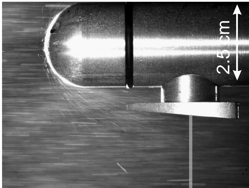
900 Figure 15. A snapshot from a high-speed video showing a flow of shattered ice fragments rebounding from the hemispherical tip of the OAP-2DC particle probe. The shattered ice fragments deflected toward the sample area (bright vertical band) are counted by the probe and artificially enhance the measured concentration. The video recording was performed in an ice spray at 80m/s in the Cox and Co. Icing Wind Tunnel Facility (for more details see Korolev et al. 905 2011, 2013ab).
