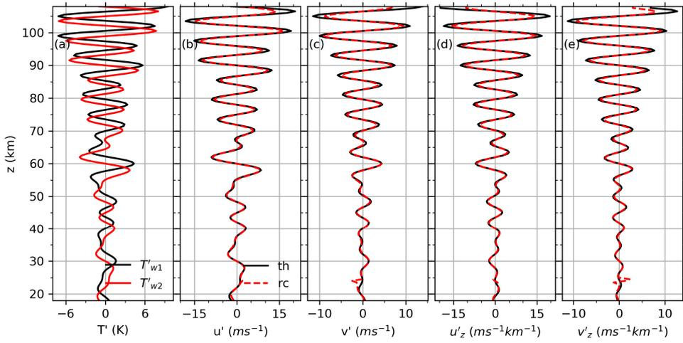
**Figure 1:** Synthetic temperature perturbation profiles (a,  $T'_{w1}(z)$  and  $T'_{w2}(z)$  are represented by black and red lines, respectively) and the corresponding winds (b, zonal; c, meridional) and shears (d, zonal; e, meridional). The winds and shears are, respectively, calculated from the prescribed amplitudes and wavenumbers (black line, labelled as “th”) and reconstructed by spectral decomposition method (red dashed line, labelled as “rc”). All panels have the same y-axis scale.
