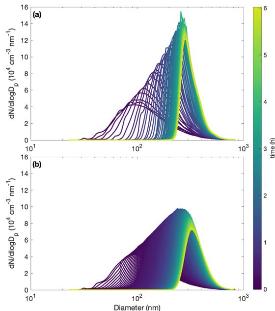
**Figure C3.** Comparison of measured (A) and simulated (B) particle size distributions throughout oxidation for experiment R1. The decay of benzyl alcohol is represented using a second-order exponential fit to the data. The accommodation coefficient of vapor to suspended particles  $\alpha_p = 1$ . Also,  $\alpha_{pw} = 0$  and  $C_w = 1 \times 10^4 \mu\text{g m}^{-3}$ . Computational time steps are taken as 1 min.
