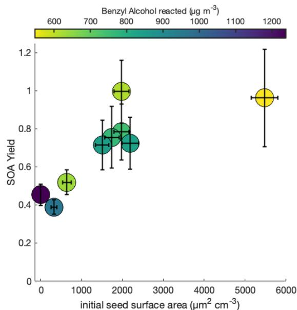
**Figure 2.** Variation in observed benzyl alcohol SOA yield with an initial NO mixing ratio of 80 ppb at 291 K as a function of the amount of benzyl alcohol reacted and the initial aerosol seed surface area. The lack of a difference in the yield over differing seed surface areas above  $\sim 1800 \mu\text{m}^2 \text{cm}^{-3}$  indicates that the experiments lie within a regime where the seed surface area does not affect the measured SOA yield.
