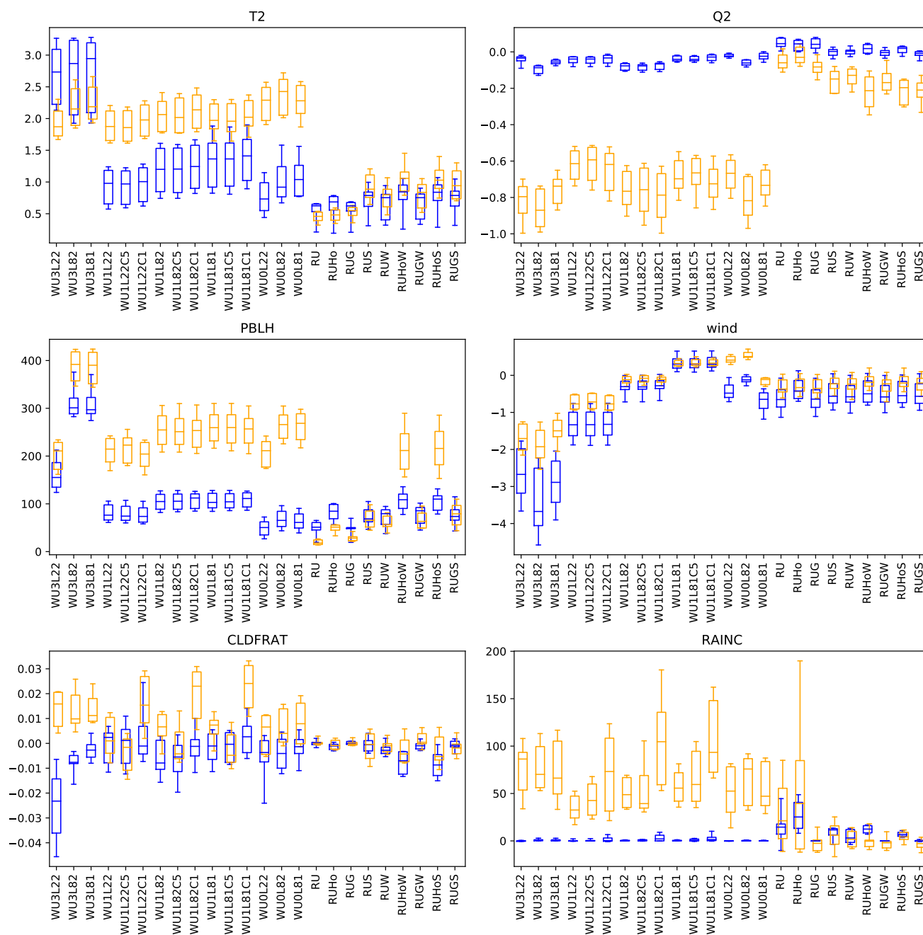
Figure 14. Winter (blue) and summer (orange) differences between city and vicinity values of 2-metre air temperature (T2; in °C), specific humidity (Q2; 10^{-3} \text{ kg kg}^{-1} ), boundary-layer height (PBLH; m), wind speed (wind; \text{m s}^{-1} ), cloud cover (CLDFRAT; fractions of one) and sub-grid scale precipitation (RAINC; mm in seasonal sums). Whiskers indicate 5th and 95th percentiles.
