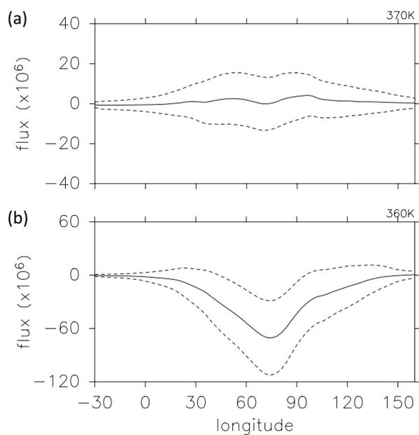
**Figure 3.** Climatological mean zonal flux of thickness-weighted low PV area as a function of longitude, calculated at the (a) 370 K and (b) 360 K isentropic levels. The unit of the flux is  $\text{kg} \cdot \text{K}^{-1} \cdot \text{s}^{-1}$ . Solid and broken lines correspond to mean values and ranges of standard deviations.
