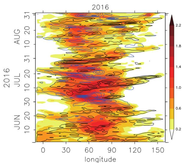
**Figure 4.** Time-longitude cross section of the air inside the AMA, defined based on the isentropic PV map. Color shadings show the thickness-weighted low PV area ( $\text{kg} \cdot \text{K}^{-1}$ ). Black and blue contours respectively show the positive and negative zonal flux of thickness-weighted low PV area. The contour interval is  $1.5 \times 10^7 \text{ kg K}^{-1} \text{ s}^{-1}$ .
