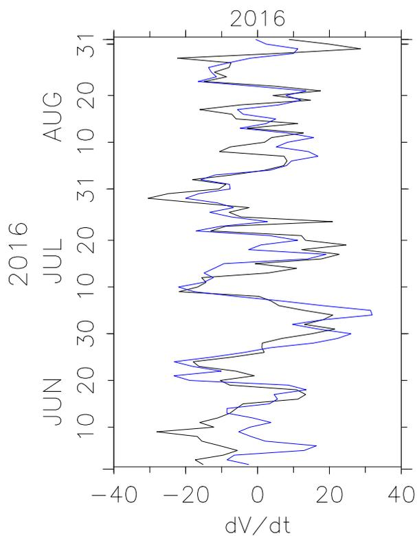
**Figure 5.** The tendency of the partial thickness-weighted anticyclone area  $\frac{d}{dt} \hat{A}_{\text{west}}$  (black: the left hand side of Eq. 4) and zonal flux  $\hat{F}$  at  $60^\circ \text{ E}$  (blue: the first term on the right hand side). The unit of the horizontal scale is  $10^6 \text{ kg} \cdot \text{K}^{-1} \text{ s}^{-1}$ .
