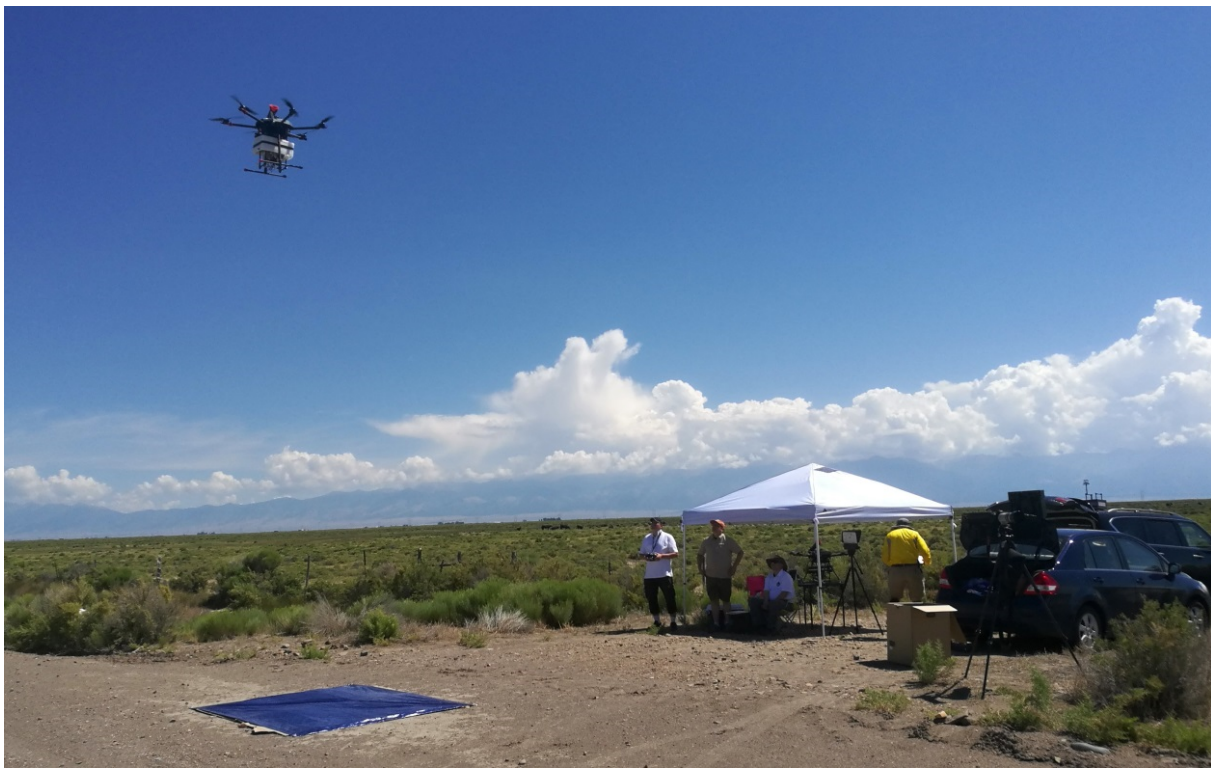
Figure 3. FMI-KSU team at dedicated spot during LAPSE-RATE campaign, gas module attached to Tarot X6 hexacopter during airborne operation. Ground module with TriSonica mini can be seen on the roof of SUV.
