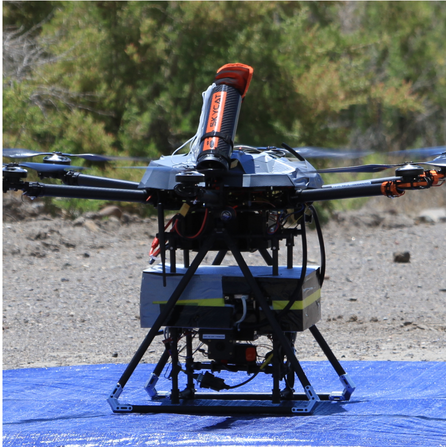
Figure 2. Particle module attached to Tarot X6 hexacopter at the take-off/landing spot - blue tarp.
