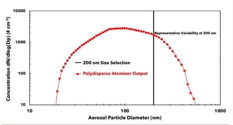
Figure S2. Atomizer size distribution and diameter of size selection. Illustrated is a typical polydisperse aerosol size distribution emanating from the atomizer prior to size selection. We size selected 200 nm diameter particles (indicated by the solid vertical black line) prior to all ice nucleation and compositional measurements. Also indicated is a standard deviation of variability in 200 nm particle concentration across all experiments.
