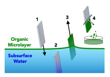
Figure S1. Sea Surface Microlayer Sampling. The plate is fully submerged below the ocean surface (1-2). The plate is then withdrawn at a slow rate (3) to allow the organically-enriched microlayer to adhere. The adhered material is scraped off (4) and the process is repeated until sufficient microlayer is collected.
