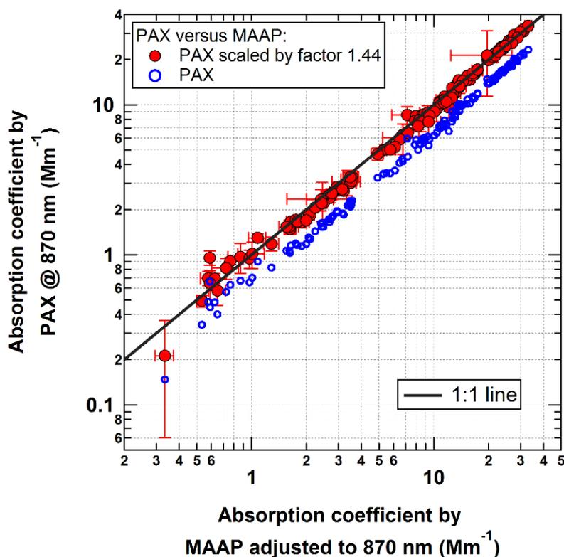
315 Figure 2. Comparison of the absorption coefficients measured by the PAX and the MAAP. The MAAP data measured at 637 nm were adjusted to 870 nm using the spectral dependence of the absorption measured by the aethalometer. The PAX data measured at 870 nm are shown with original calibration and after scaling by a factor 1.44 to match the MAAP data on average.
