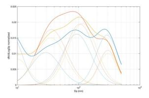
Fig. R5 Normalized size distributions in blue: arctic mesocosms, yellow: Mediterranean ship and orange: NZ coastal mesocosms. Bold line are for the full size decomposition and light lines for their mode decomposition. Sellegri et al., (2020)
