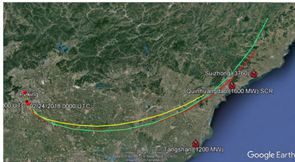
Fig. 1. Fig. 1: HYSPLIT 12 h backtrajectories for 24022018 01:00 UTC arrival in Beijing, yellow 50 m, red 250 m and green 500 m, GDAS 0.5
