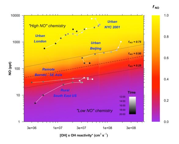
520 Figure 3: Variation of the fraction of ISOPOO reacting with NO as a function of NO concentration and the reactivity of the system. The plot is derived from a series of zero-dimensional box model runs performed as a function of fixed concentrations of [NO], [OH], and [isoprene]. Photolysis is fixed to an average of 09:00-17:00 conditions. OH reactivity\* is total OH reactivity of the chemical system minus the contribution from OH + NOx (Equation E1), since these reactions do not produce RO2.
