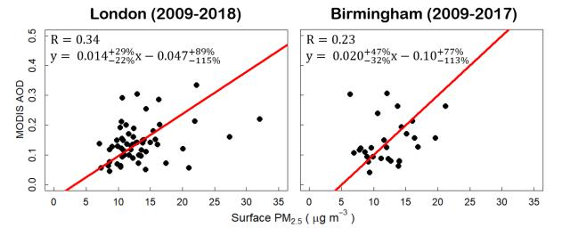
Figure 4 Assessment of MODIS AOD with surface PM<sub>2.5</sub> in London and Birmingham. Points are monthly means of city-average AOD from MODIS and PM<sub>2.5</sub> from surface networks for London (left) and Birmingham (right). The red line is the SMA regression.
