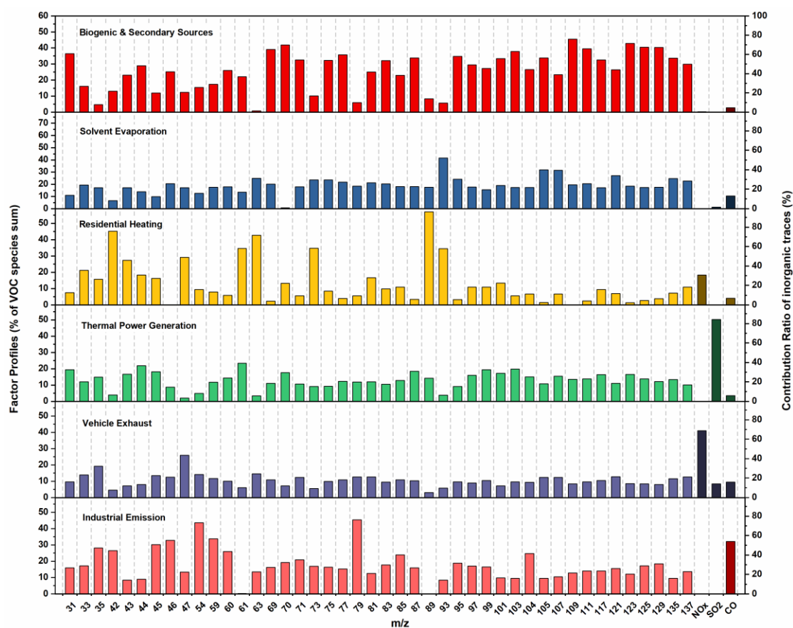
Figure S7. Factor profiles of major emission sources resolved by the positive matrix factorization (PMF) model. The bright columns represent VOC profiles corresponding to the left Y-axis, and the dark columns represent inorganic tracer profiles corresponding to the right Y-axis.
