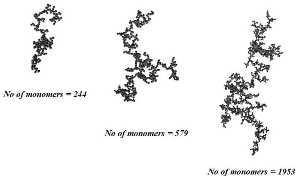
Figure 3: Fractal model morphologies composed of different number of monomers, used in MSTM code. For all fractals we use the same fixed value of fractal dimension D_f and fractal pre-factor k_f .
