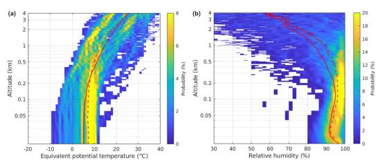
Figure 7: Probability of (a) equivalent potential temperature and (b) RHw as a function of altitude. Note that the probability is calculated for each height; hence, for each layer the probability sums to 100%. The red solid line shows the mean and the red dashed line the median profile.
