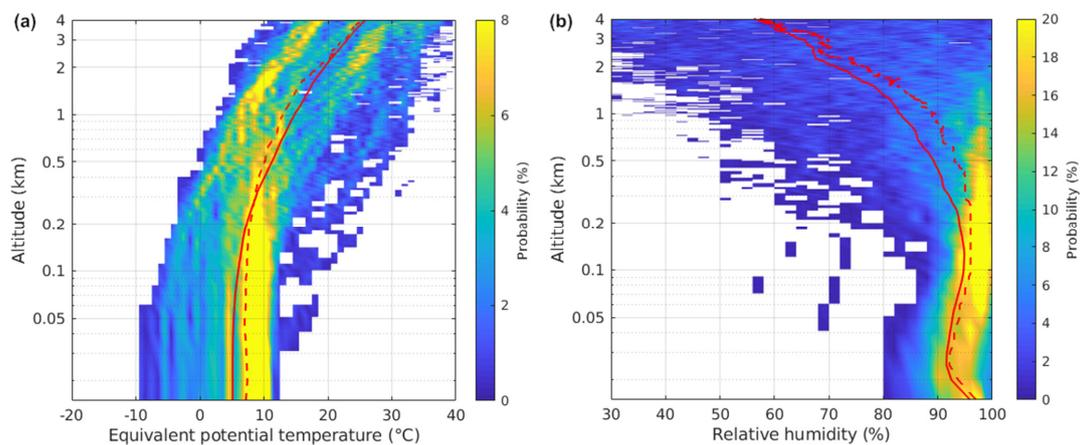
**Figure 7: Probability of (a) equivalent potential temperature and (b) RHw as a function of altitude. Note that the probability is calculated for each height; hence, for each layer the probability sums to 100%. The red solid line shows the mean and the red dashed line the median profile.**
