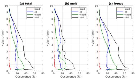
Figure 10: Mean cloud occurrence per volume for different cloud types, obtained from the Cloudnet target classification product: (a) mean profiles for all available Cloudnet data, (b) for the melt period, and (c) for the freeze period.
