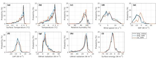
Figure 5: Probability distributions of (a) surface temperature, (b) near-surface air temperature, (c) RHw, (d) wind speed, (e) sensible heat flux, (f) latent heat flux, (g) shortwave net radiation, (h) longwave net radiation, and (i) surface energy. Data are from measurements on board the ship for the whole measurement period (black lines), for the ice drift period only (blue line), and from the measurement station on the ice floe (orange line).
