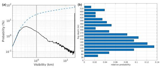
Figure 9: (a) Probability distribution and accumulated probability (blue dashed line) of visibility. The black vertical line marks 1 km visibility. (b) Probability distribution of fog depths detected using radar RHI scans.
