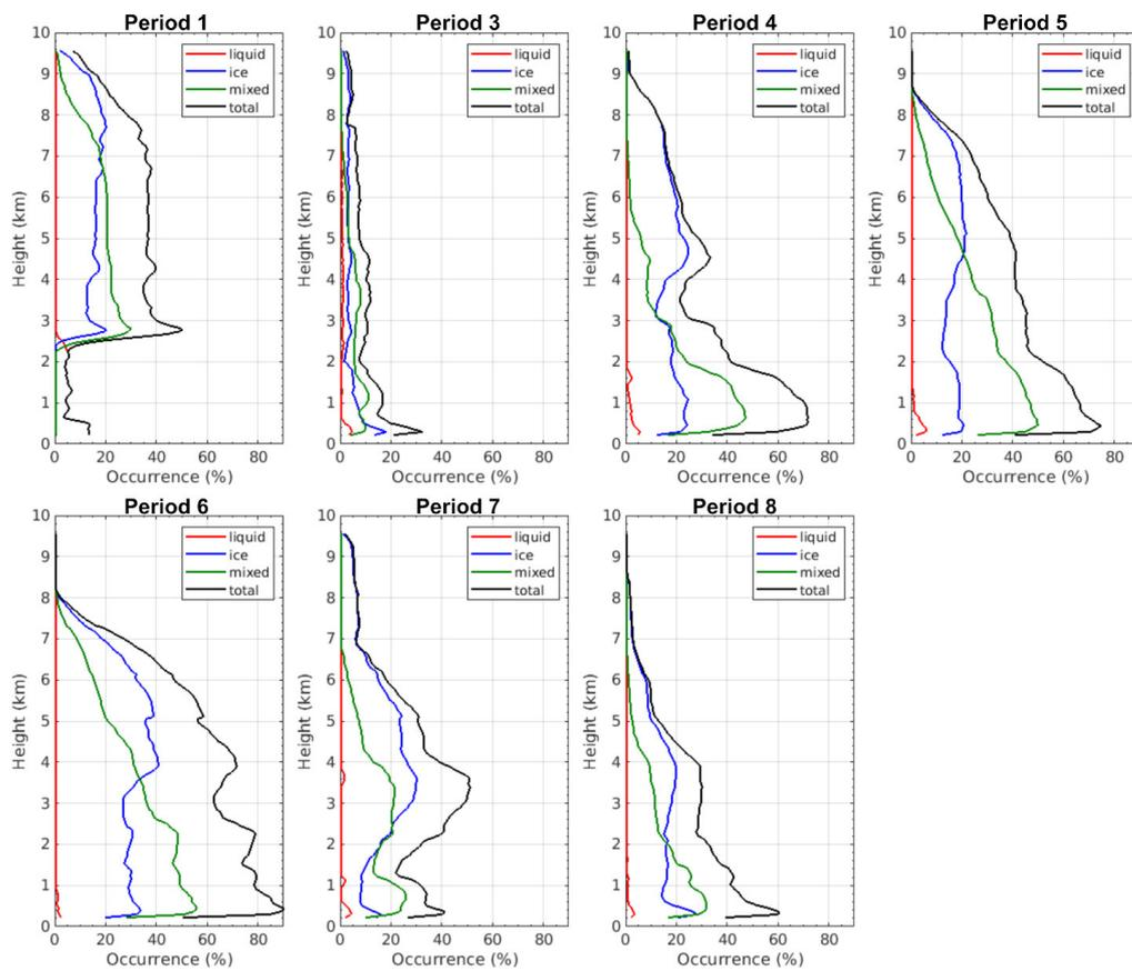
**Figure 15:** Mean cloud occurrence per volume for different cloud types (colour coded), obtained from the Cloudnet target classification product for the eight key periods.
