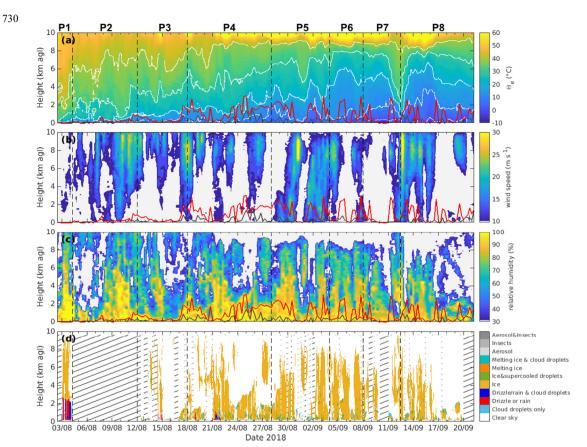
Figure 6: Contour plots of (a) equivalent potential temperature, (b) wind speed, (c) RHw measured by radiosondes, and (d) cloud target classification from the Cloudnet algorithm. The red lines in (a)-(c) show the main inversion base height and the grey lines the surface mixed layer depth identified from radiosonde data. Dashed vertical lines mark the identified key periods.
