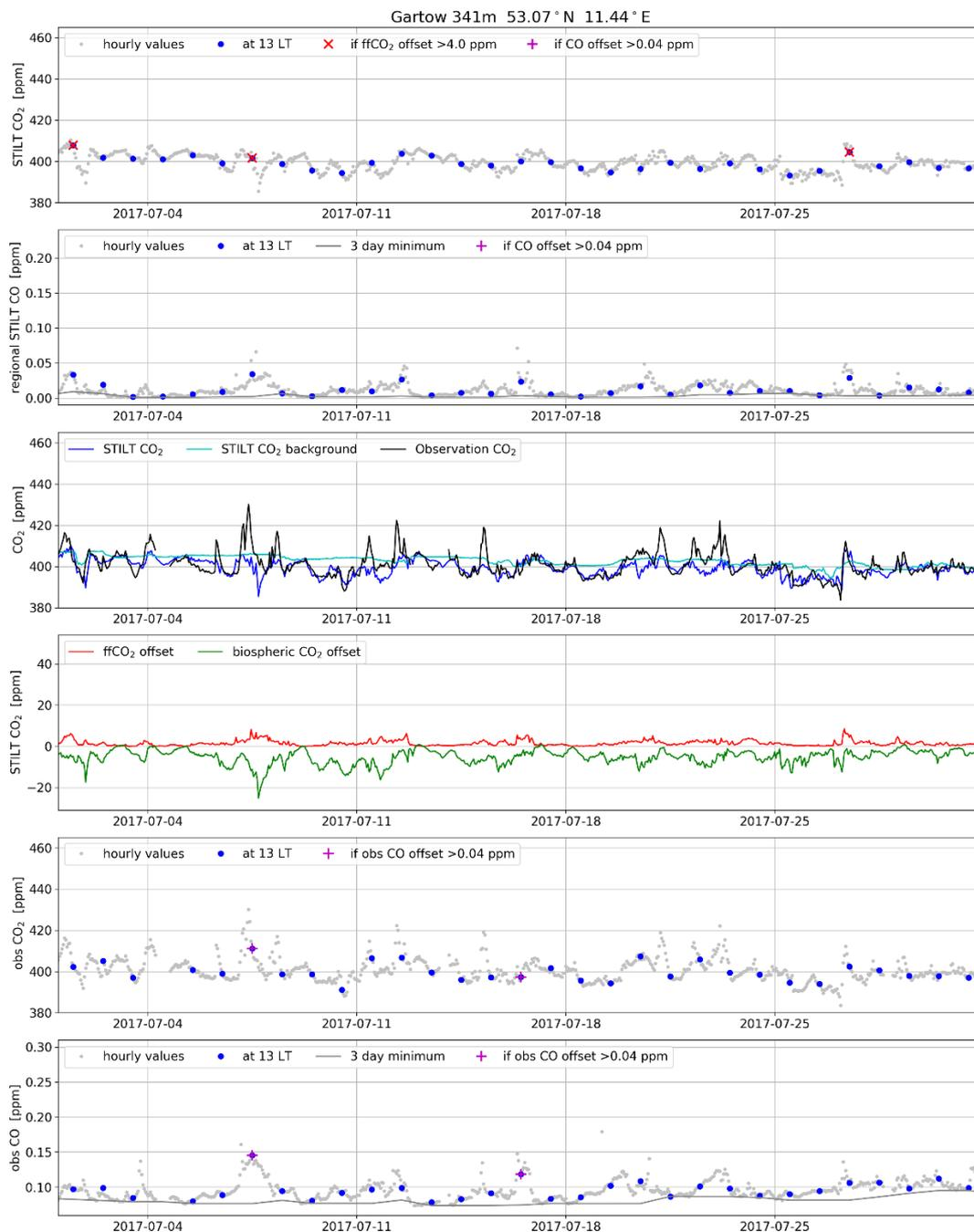
740 **Figure 8:** Variability of STILT-simulated (upper four panels) and measured (lower two panels) CO<sub>2</sub> and CO concentrations at
