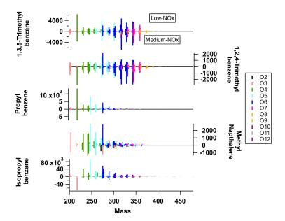
Figure 2 Average mass spectra of particle phase measurements from I-CIMS for all precursors under low-NOx conditions (upwards) and medium-NOx conditions (downwards – negative values correspond to magnitude of positive signal)
