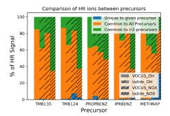
390 Figure 6 Comparison of signal contributions of ions which were commonly observed from all precursors (orange), ions common to two or more precursors (green) and ions unique to the given precursor (blue) for all precursors and experiments
