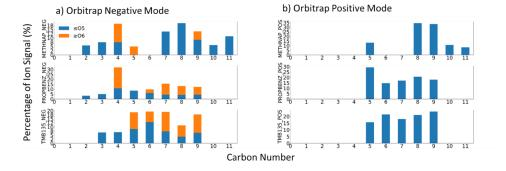
Figure 4 Signal distribution across carbon number coloured by proportion of HOM signal for a) Orbitrap Negative mode and b) Orbitrap Positive Mode [only signal contributions up to precursor carbon number are included (C<sub>9</sub> for TMB135 and PROPBENZ, C<sub>11</sub> for METHNAP) capturing relevant products for mechanistic discussions below. Ions which contributed less than 0.5 % of observed signal were assumed to be background and removed.]
