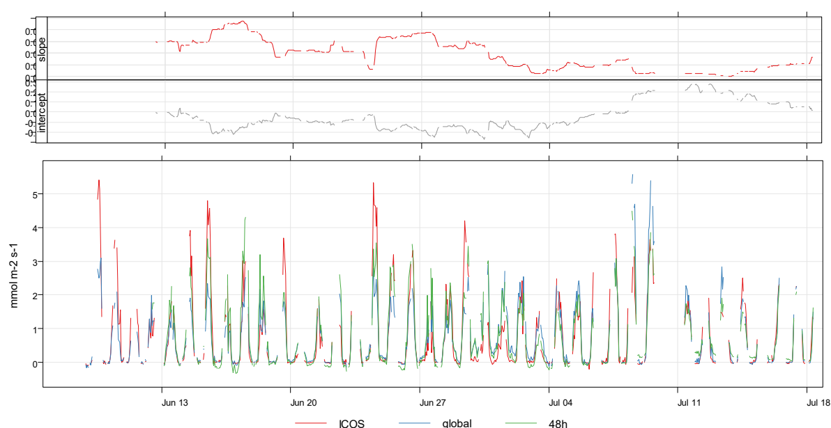
Figure S7. Bottom graph: water vapour flux as measured at ICOS, and the PTRMS either calibrated over the entire period or over rolling 48 h. The slope and intercepts of the rolling calibration are also given in the top graph.
